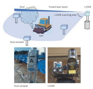
"LIDAR" is a technology to measure the distribution of dust using harmless lasers.
