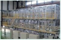
Continuous hydrogen production test facility made of H<sub>2</sub> production rate: up to 0.1m<sup>3</sup>/h-H<sub>2</sub> Size: W18.5×D5×H8.1 (m)
