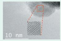
TEM image of hillock in BaF<sub>2</sub> formed by heavy ion irradiation
